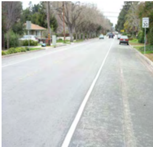
Middle Avenue is too narrow to provide for both on-street parking and a bike lane; however, the relatively wide shoulder/parking area provides adequate width for a Class III bicycle route.
