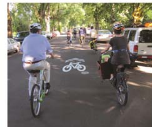
Sharrows help confirm routes and guide cyclists on Class III facilities
