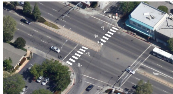
Matadero/Margarita Avenue at El Camino Real. The slightly off-set nature of this intersection creates excessively long and/or out-of-direction crossings. Creative measures to improve the geometry and visibility of this crossing (potential example above right) are needed in order to develop the high priority Matadero-Margarita Bicycle Boulevard.
