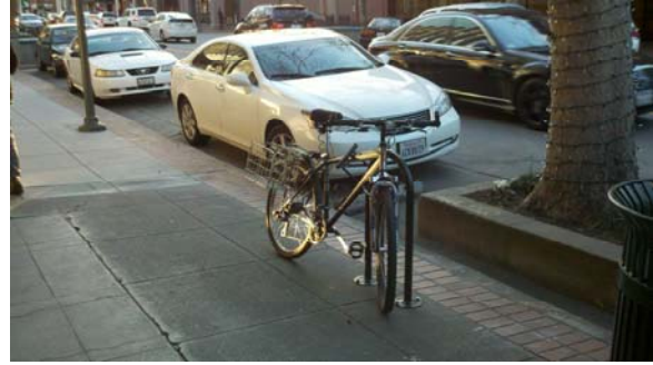
A conventional inverted-U style rack supports the bicycle on two points of contact and provides easy-to use bicycle parking.
