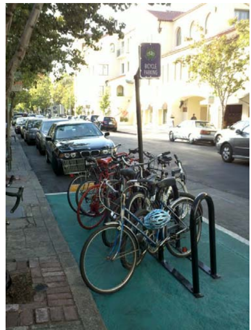
The on-street bicycle parking “corral” at the Coupa Café provides bicycle parking without impeding the sidewalk for pedestrians.
