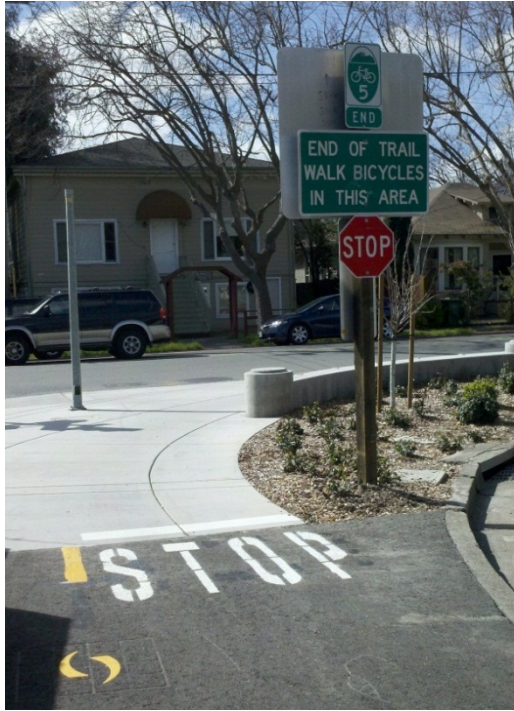
(Above): Shared use path and roadway intersection with “cross bike” pavement markings and pedestrian lighting – Ohlone Greenway, Berkeley, CA. (Left): Urban trailhead, San Rafael, CA. Note high visibility signage, a lack of unnecessary barriers, and inclusion of a “mixing zone” gateway feature as elements of this successful path terminus.
