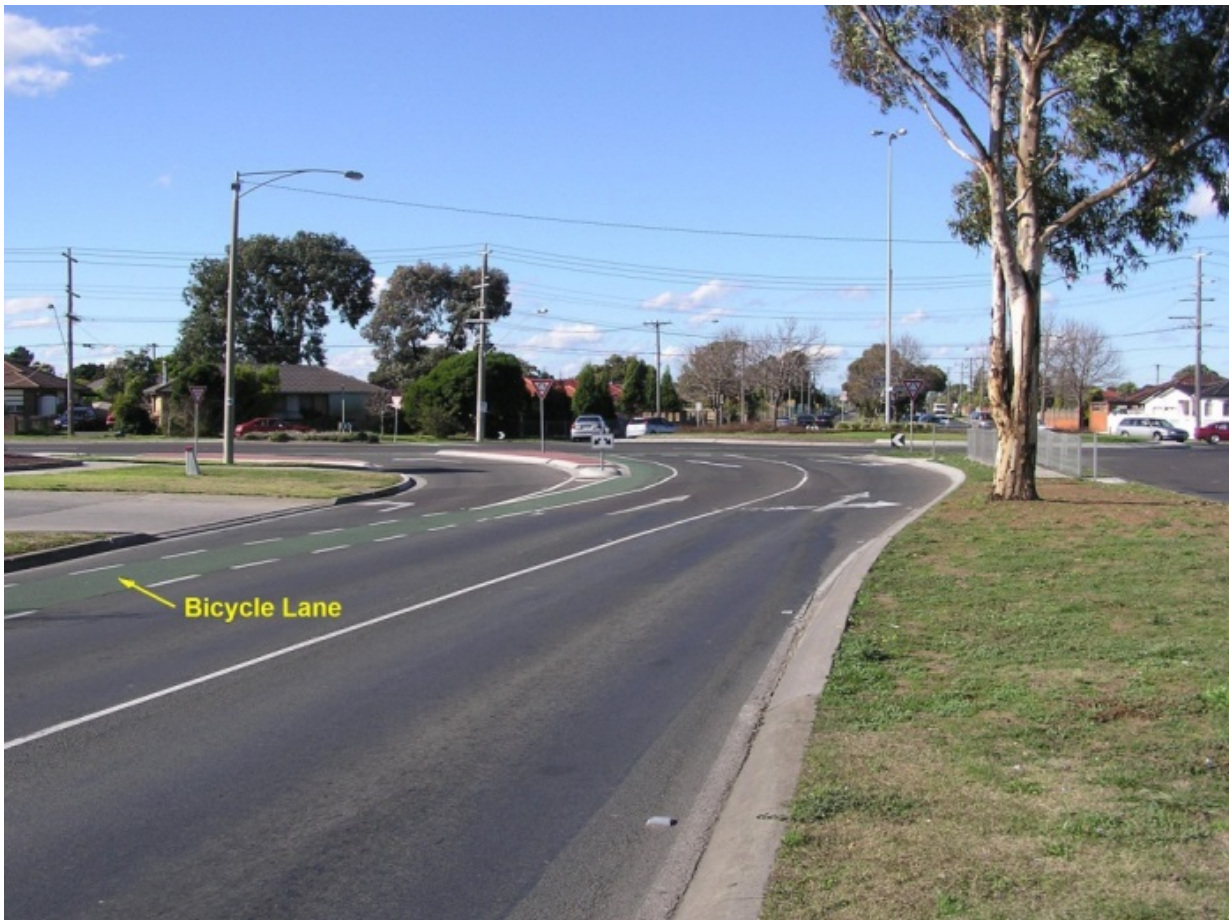
Figure 5.19: Bicycle lane continuing past a left-turn slip lane at a roundabout (some jurisdictions may not favour this treatment – see previous text in this Section)
