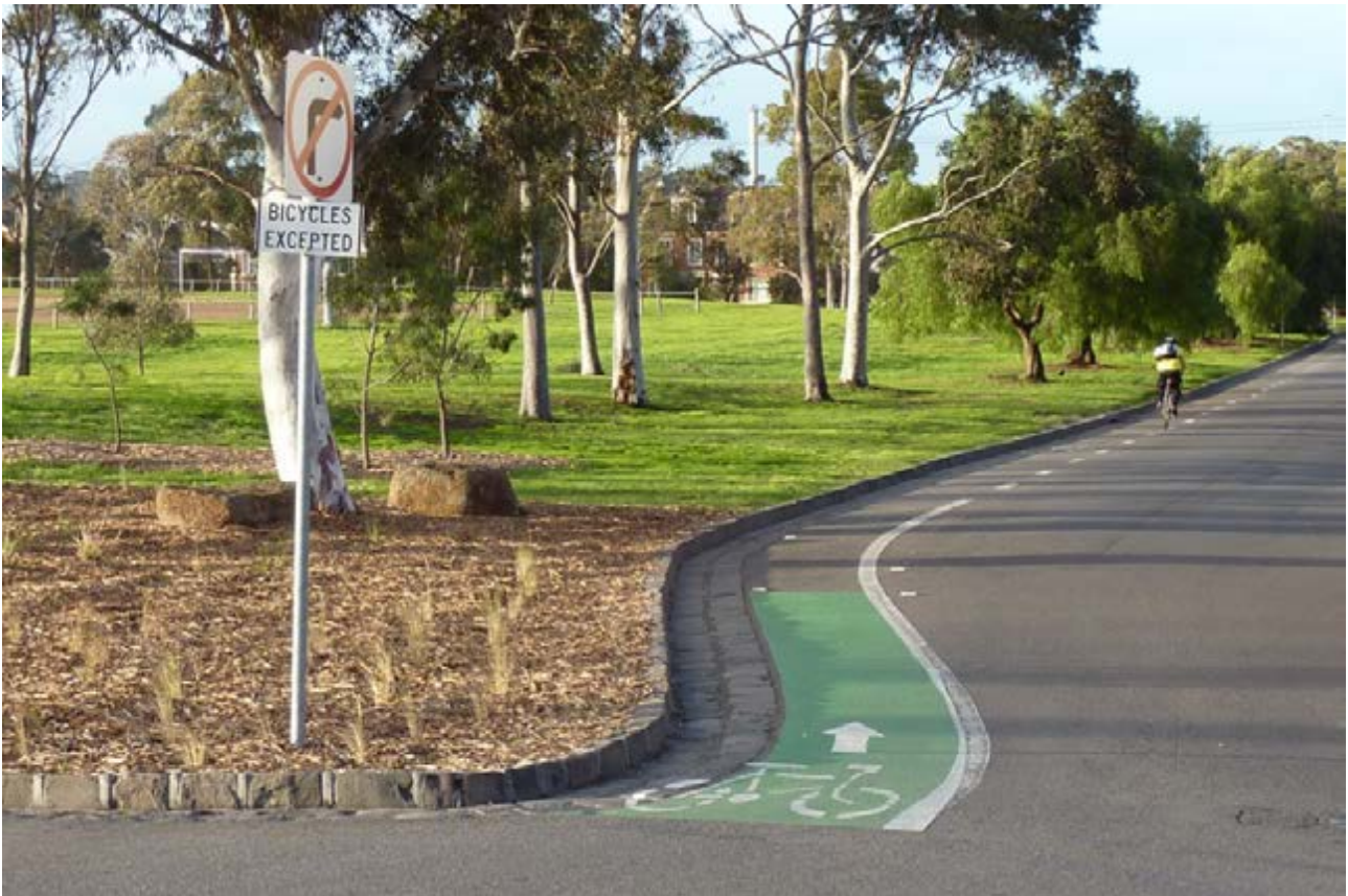
Figure 4.5: Contra-flow bicycle lane example
